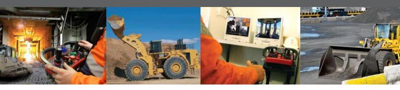
Loader operators are often required to operate in unstable or high risk environments. RCT can convert loaders to remote control which removes the operator from the driver seat - enabling them to tackle the more hazardous tasks without the risk of injury; making them more confident and productive. RCT remote control solutions allow remote operation of loaders from a distance away with greater overall vision of the surrounding work area. Business risk is managed and production continues.
