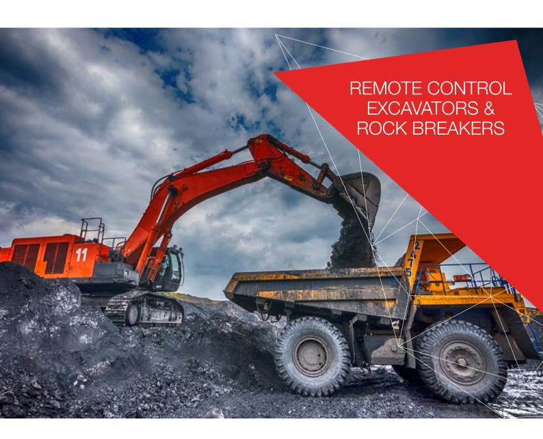
RCT has successfully placed a number of excavators/rock breakers on remote control. The ControlMaster® control options range from Line-of-Sight, Teleremote to Automation, placing operators at a safe location away from the hazardous area. ControlMaster®
